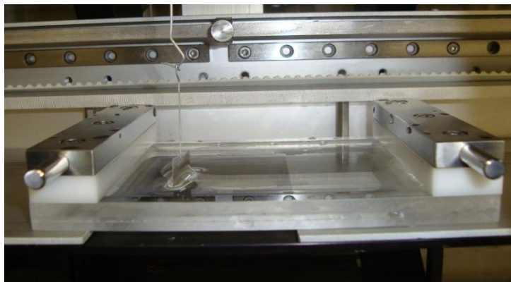
Figure 3-1. The area of the PMMA trough was reduced using Delrin barriers and the surface pressure at each surface area reduction was measured using the Wilhelmy plate setup.
